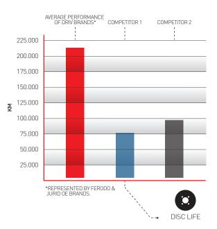
Measurements performed by Applus IDIADA. Test conducted on a dyno (test bench) simulating the vehicle conditions. Shown is the average expected lifetime after final measurements over a 2018km mileage, comparison between a total of 4 manufacturers using one disc/pad set each.
