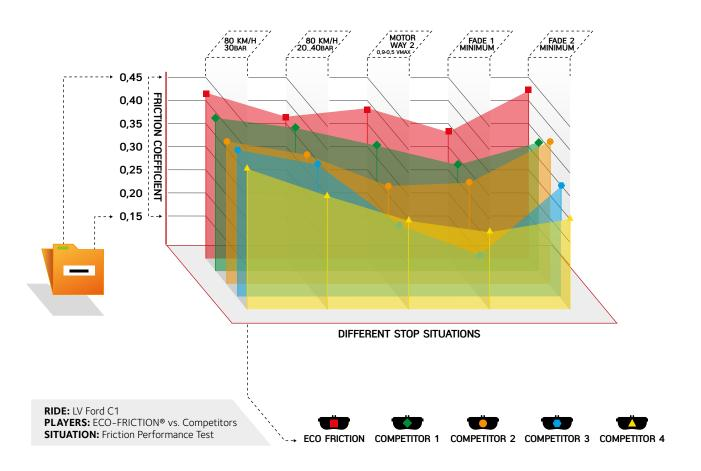
Consistency is key. To keep control, and to be one step ahead of whatever's in front of you. Test results show that ECO-FRICTION® Brake Pads not only provide powerful stopping power, their performance remained stable throughout all situations, from varying speed settings to extreme temperatures.
